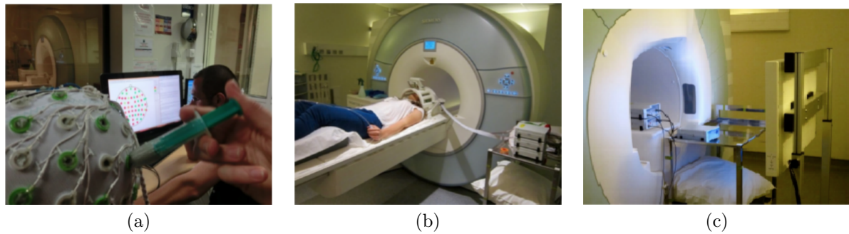
Figure 23: Reproduced from Mathis Fleury's thesis: preparation of a simultaneous EEG-MRI-NF session with a 3T MRI and a 64 electrodes EEG cap, at the Neurinfo imaging platform. (a) Installation of the EEG subsystem and verification of impedance outside the MR environment, (b) Installation of the MR coil and rechecking of the EEG impedance, (c) Placement of the amplifiers, battery and LCD screen to display the visual feedback.
