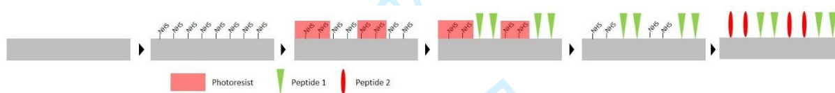
Figure 2. Scheme of preparation of the pattern surfaces
