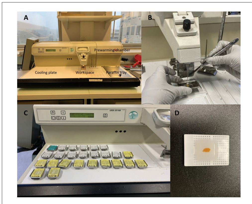
Figure 2 Paraffin embedding process of embryonic mouse tissue. (A) The paraffin embedding process is a manual process taking place using a tissue embedding system. (B) The brain tissue is appropriately placed in the center of the metal mold filled with melted paraffin embedding medium using the heated paraffin dispensing system of the station. The base of the original cassette is then immediately placed on top of the mold. (C) The mold is placed on the cooling unit set at -5^{\circ}\text{C} , allowing the paraffin to solidify. (D) The formed paraffin block is removed from the mold.
