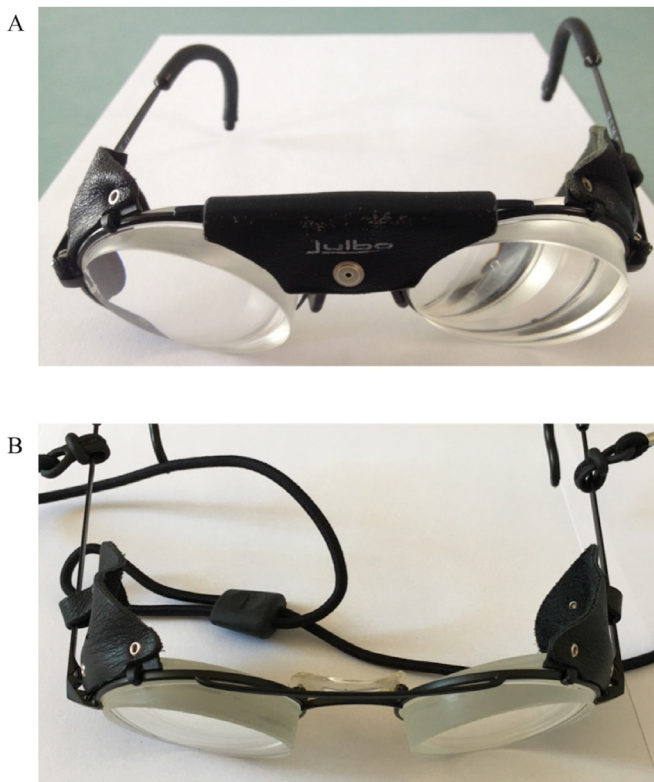
Figure 2 Prismatic glasses (A) and sham glasses (B). (A) A pair of prismatic glasses with an optical deviation of 10 degrees towards to the right side; (B) a pair of sham glasses with a neutral optical deviation.
