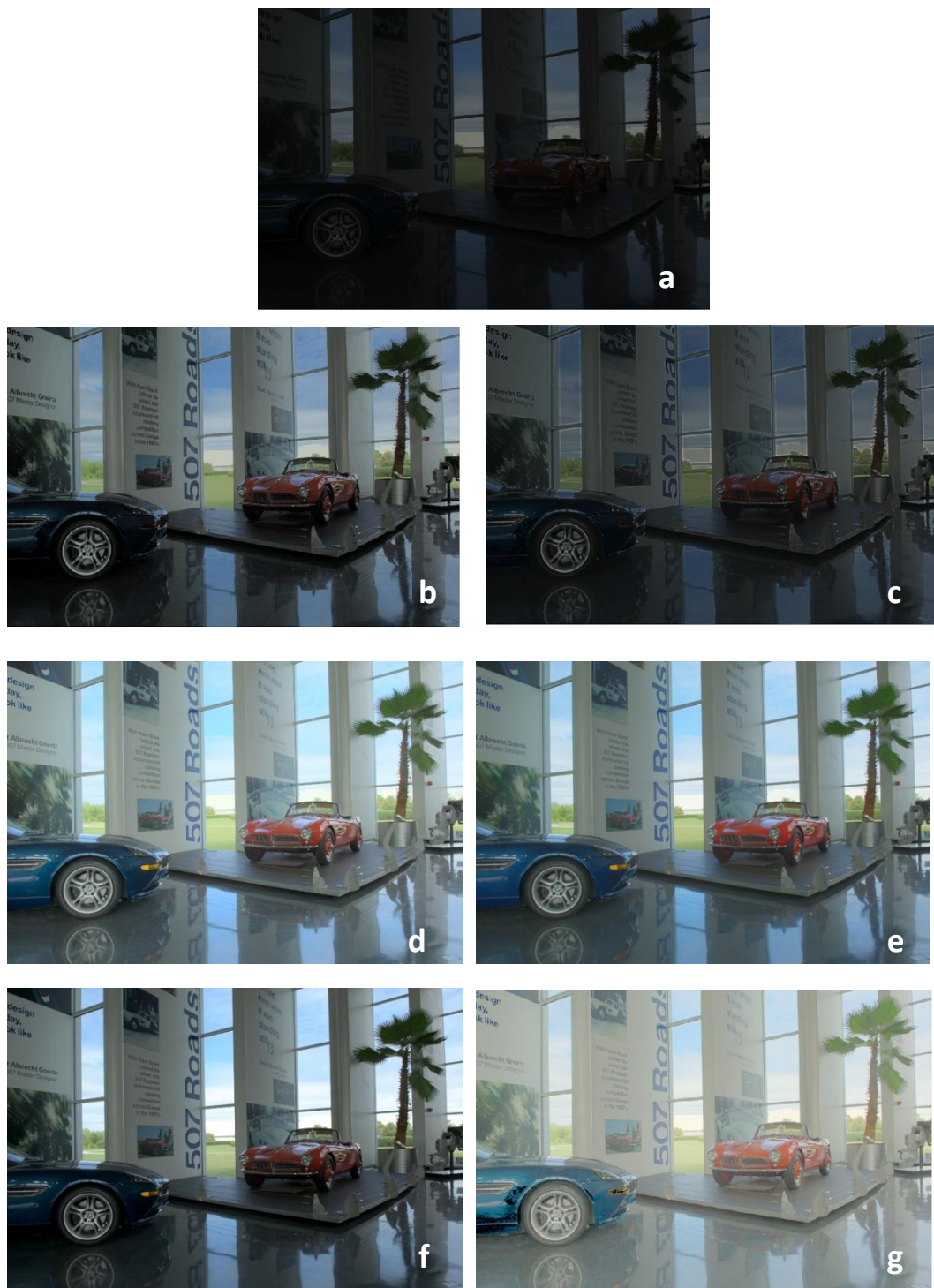
Figure 8 Comparison of the proposed algorithm with different image enhancement methods. (a) Original image from [22], (b) result of the proposed algorithm without the retina-like filtering, (c) result of the proposed algorithm with the retina-like filtering, (d) result of the Drago operator, (e) result of the Reinhard operator, (f) result of the Mantiuk operator, (g) result of the Retinex operator.
