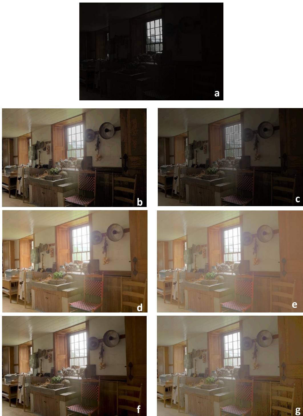
Figure 7 Comparison of the proposed algorithm with different image enhancement methods. (a) Original image from [22], (b) result of the proposed algorithm without the retina-like filtering, (c) result of the proposed algorithm with the retina-like filtering, (d) result of the Drago operator, (e) result of the Reinhard operator, (f) result of the Mantiuk operator, (g) result of the Retinex operator.
