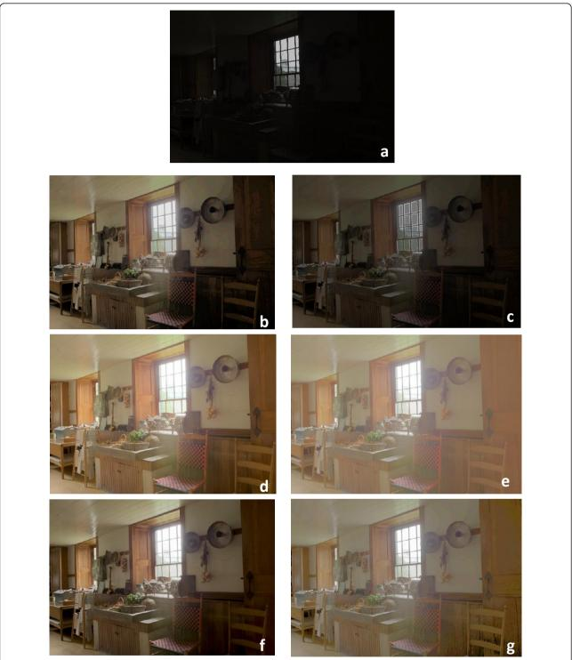
Figure 7 Comparison of the proposed algorithm with different image enhancement methods. (a) Original image from [22], (b) result of the proposed algorithm without the retina-like filtering, (c) result of the proposed algorithm with the retina-like filtering, (d) result of the Drago operator, (e) result of the Reinhard operator, (f) result of the Mantiuk operator, (g) result of the Retinex operator.
