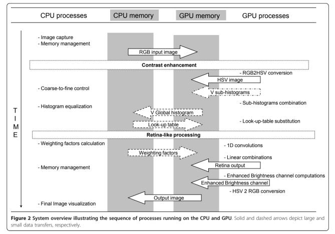
convolution operator. Therefore, we can reduce the processing only to the convolution of each color channel with two different Gaussian masks. Then, these filtered channels are linearly combined. Equations (16) to (18) describe mathematically this simplification:
