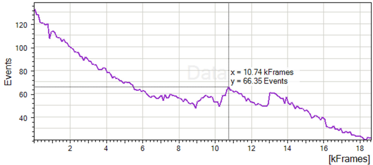
Figure 3. Typical histogram of the number of localizations per frame for the Alexa Fluor-647 dye. The curve is built using blocks of 100 frames each for smoothing reasons. Note increases in the number of localizations (middle part of the graph) due to an increase in intensity of the “backpumping” 405 nm laser. Exposure time is 50 ms/frame, detection threshold is 80 photons/pixel; 18620 frames with 1161303 events were analyzed. The analysis was done in the Leica LAS AF software.
