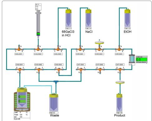
**Fig. 2** Overview of the automated synthesis cassette for radiolabelling of PSMA-11. This figure was obtained from Thisgaard et al. (2021) which was licensed under a Creative Commons License http://creativecommons.org/licences/by/4.0/
