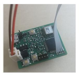
FIGURE 9. Prototype V2 (Bluetooth): integrated final electronic board.
