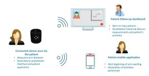
FIGURE 4. Lymphometer acquisition and treatment system.
