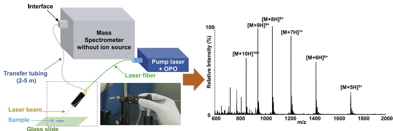
FIG. 1. Schematic representation of the Remote IR-MALDI prototype so-called SpiderMass system. The system is composed of three parts including a fibered laser tuned to 2.94  $\mu\text{m}$  equipped with a hand-piece for maneuvering the laser beam onto surfaces, a Tygon® ND 100–65 transfer tubing line connected to the laser hand-piece on one end and to the inlet of the MS instrument on the other, and the MS instrument itself (here an Ion mobility QqTOF).
