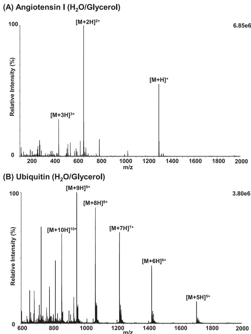
FIG. 2. MS spectra recorded in positive mode using the Re-AP-IR-MALDI system for (A) angiotensin-I and (B) bovine ubiquitin in water/glycerol (1:1, v/v) as matrix. 2  $\mu$ l of analyte at  $5 \times 10^{-4}$  M was deposited onto a glass slide and submitted to 5 s laser irradiation period (ca. 50 laser shots).
