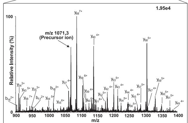
FIG. 4. MS<sup>2</sup> spectrum of the precursor ion [M+7H]<sup>7+</sup> ( $m/z$  1224.4) and [M+8H]<sup>8+</sup> ( $m/z$  1071.3) of bovine ubiquitin recorded in real-time in positive mode using the SpiderMass prototype. 2  $\mu$ l of analyte at  $5 \times 10^{-4}$  M was deposited onto a glass slide and submitted to 5s laser irradiation period (ca. 50 laser shots).
