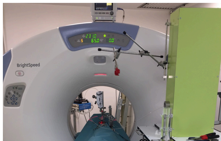
Fig 1. Preclinical injection system developed by EVEON. The injector is located beside the operation table in CT room. The injection needle is connected to the injector through a connection tube to transfer the Ho suspension from the injector to the needle.
