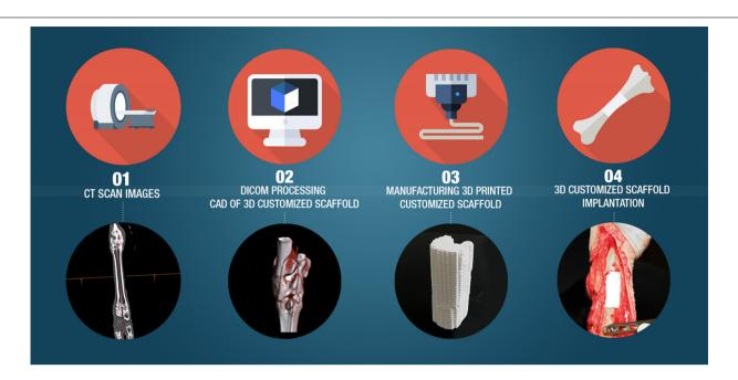
FIGURE 3 | Workflow involved in customizable bone construct fabrication. (1) CT scans of the patient's bone are acquired. (2) Computer aided software enables the processing of CT images in order to (3) 3D print personalized scaffolds for (4) bone defect reconstruction. The lower panel illustrates a real large bone defect reconstruction in a sheep metatarsal bone model.
