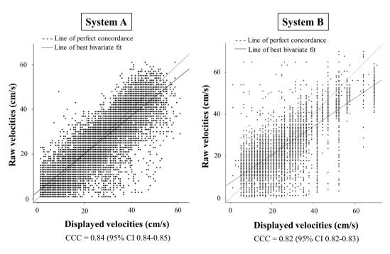
**Figure 5.** Lin's concordance correlation coefficient (CCC) between the pixel-to-pixel velocity value comparison extracted from the raw proprietary velocity data and the displayed velocity data estimated from the look-up table, on one sample of color-Doppler M-mode acquisition for both systems A and B. The line of perfect concordance is the line of identity (y = x); the reduced major axis corresponds to the regression line between the two measurements.
