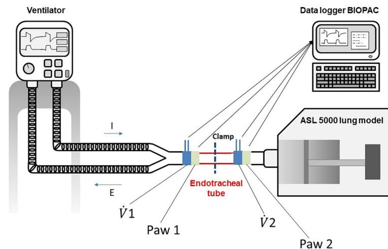
**Fig 1. Experimental set up.**  $\dot{V}1$  = flow measured with pneumotachograph number 1,  $\dot{V}2$  = flow measured with pneumotachograph number 2, Paw 1 = pressure measured with pressure transducer number 1, Paw 2 = pressure measured with pressure transducer number 2. Arrows indicate the connection between Paw ports and flow meters to data logger. The location of the clamp into the endotracheal tube is shown. I = inspiration, E = expiration.
