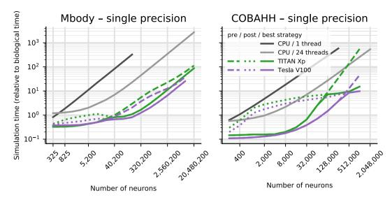
**Figure 1.** Benchmark of the net simulation time on a 12 core CPU with a single thread (dark gray) or using OpenMP with 24 threads (light gray), compared to a consumer GPU (TITAN Xp) and an HPC model (Tesla V100). For the GPUs, simulation times are displayed separately for a pre-synaptic parallelisation strategy (dotted) or post-synaptic strategy (dashed). The better of the two strategies is highlighted by a solid line.
