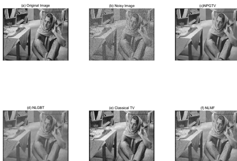
Fig 6. Results of different denoising methods on 576x720 Barbara image. The image is corrupted by the noise at \sigma = 30\text{ dB} . (a): Original image. (b): Noisy image. (c): NPGTV with k = 5 , \lambda = 0.05 , patch size 9 \times 9 . (d): NLGBT algorithm. (e): Classical TV. (f) NLMF with search window size 3 \times 3 , similar widow size 5 \times 5 and the standard deviation is set to 0.1. (The original Barbara image in our paper is taken from Fig 1 in [19] published by the journal PLOS one, which is licensed under the Creative Commons Attribution International License (CC BY 4.0)).
