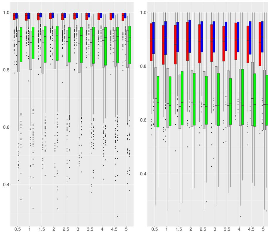
**Fig. 6** AUC for SegCorr and TCM (Scenario 3). AUC of the SegCorr ( $n = 50$ -red,  $n = 100$ -blue) and TCM ( $n = 50$ -grey,  $n = 100$ -green) algorithms for Scenario 3 as a function of  $\beta$ . *Left: gene level. Right: region level*
