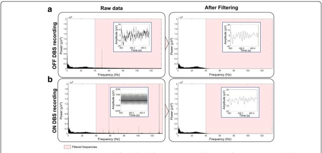
**Fig. 1** Power spectrum and EEG time series at rest before (left) and after (right) correction of the DBS artefact. **a** With DBS turned OFF. **b** with DBS turned ON. The EEG recording was obtained in a PD patient stimulated at 130 Hz bilaterally in the STN. A low pass filter with a cut-off at 40 Hz was applied to remove the DBS artefact. See (Kibleur et al. 2016) for full description of the data acquisition procedure
