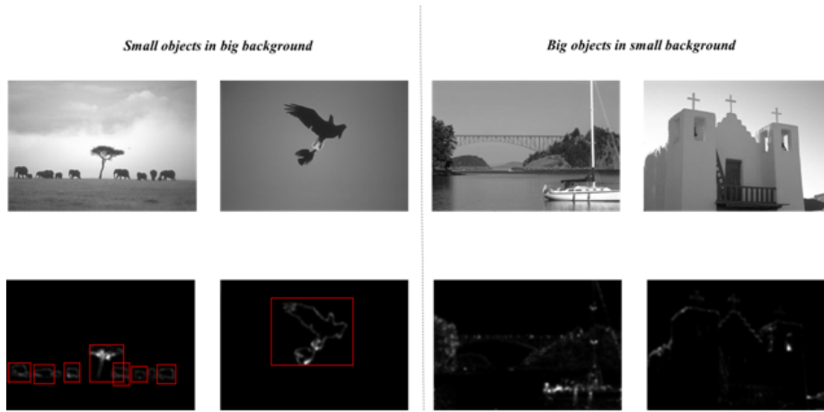
Fig. 2 . Proto-objects extraction based on saliency map.
