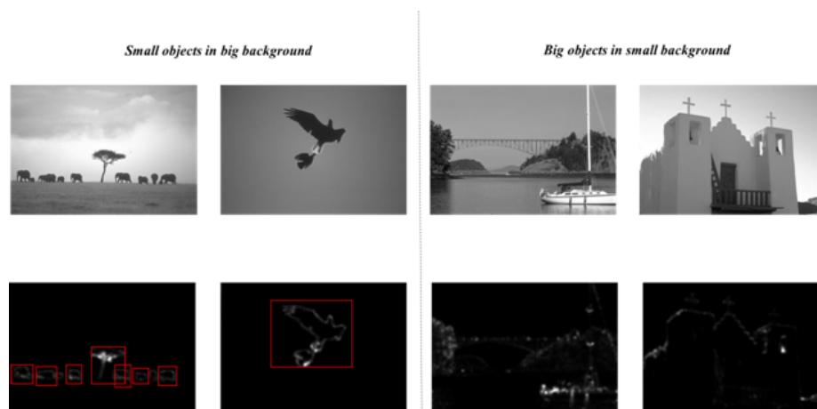
Fig. 2 . Proto-objects extraction based on saliency map.
