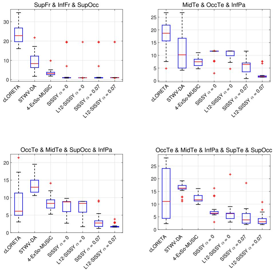
Figure 4: Boxplots of Dipole Localization Error (DLE) results (the lower the better) of the tested source imaging algorithms for 4 different multi-patch scenarios and 50 realizations with different signals and background activity.
