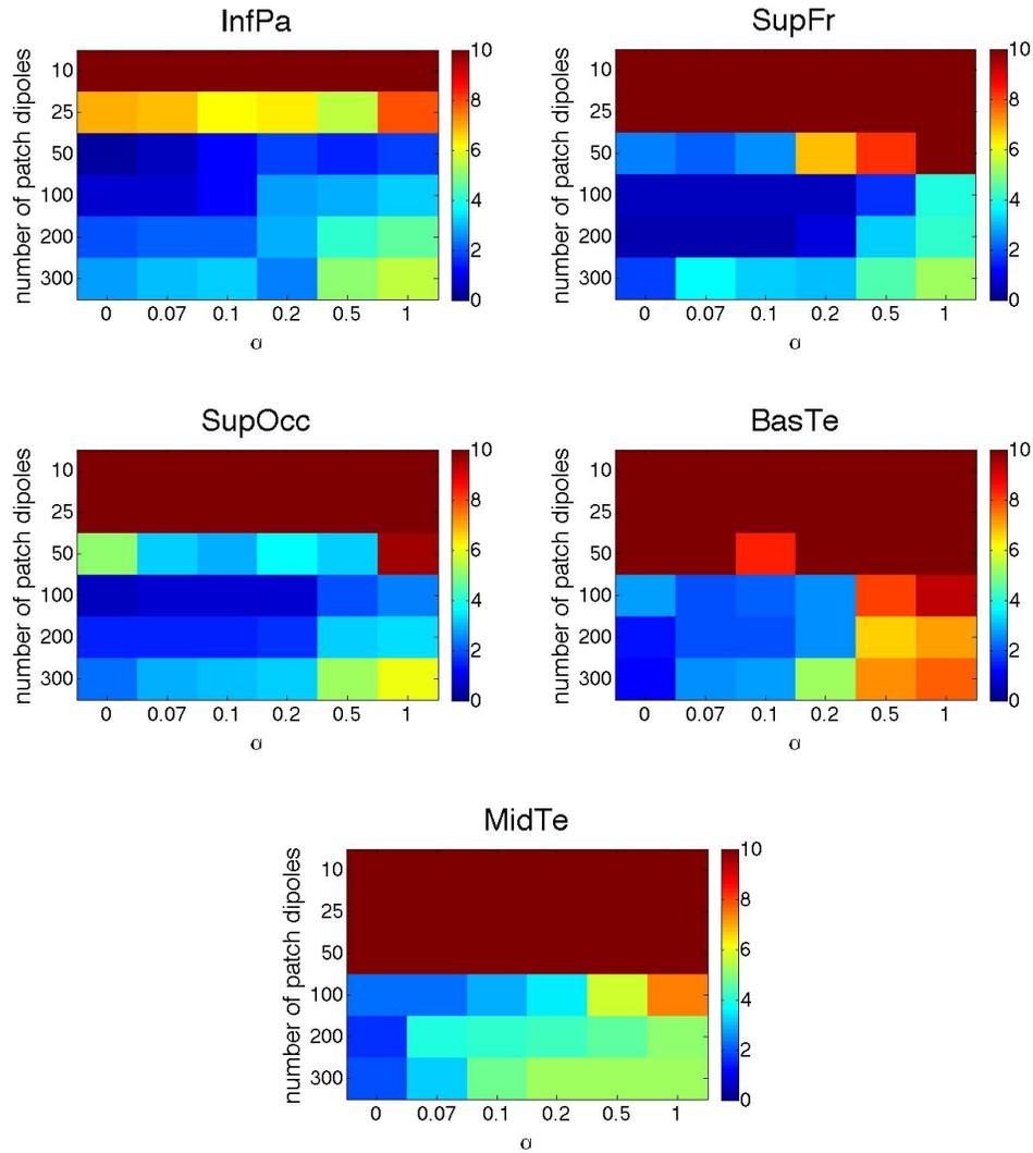
Figure 2: Dipole Localization Error (DLE) coded in color (the smaller (blue) the better) for different patch positions depending on the patch size and the regularization parameter  $\alpha$ . Note that the upper limit of the DLE has been fixed to 10 mm, meaning that DLE values higher than this threshold have been replaced by 10 mm.
