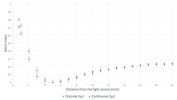
Figure 7. First-order Sobol indices ( $S\mu s$ ') computed with two different analytical equations (discrete and continuous method) for different distances from the light source. These Sobol indices quantify the contribution of the analytical model's variance to the effect of reduced scattering coefficient variation.
