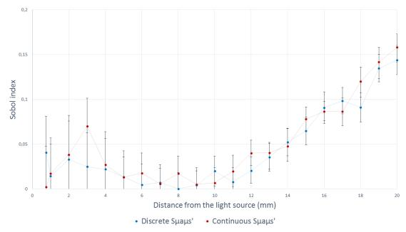
Figure 8. Second-order Sobol indices (Sμaμs' and Sμaμs') computed with two different analytical equations (discrete and continuous method) for different distances to the light source. These Sobol indices quantify the sensitivity of the analytical model's variance to the interaction of reduced scattering and absorption coefficients variations.
