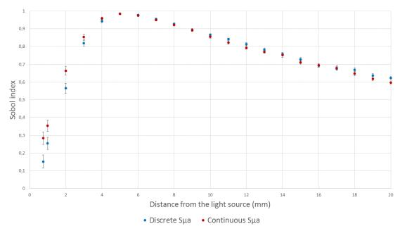
Figure 6. First-order Sobol indices ( $S\mu a$ ) computed with two different analytical equations (discrete and continuous method) for different distances to the light source. These Sobol indices quantify the contribution to the analytical model's variance to the effect of absorption coefficient variation.
