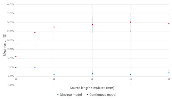
Figure 5 Data points are the mean relative deviations of fluence rate values computed by discrete and continuous methods, calculated for all six different source lengths over each distance d (0.75 mm to 10 mm). Error bars are standard deviations.
