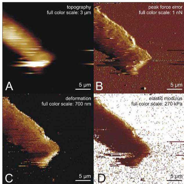
**FIGURE 2.** Peak-Force quantitative nano-mechanical (PF-QNM) measurements on a lens cortical cell. At each pixel of the image, a force-distance curve was acquired from which the different parameters were extracted. Topography (A), peak force error signal (B) deformation map (C), and elasticity map (D) were measured concomitantly. The bright area in D corresponds to the hard glass substrate resulting in saturation in the stiffness signal.
