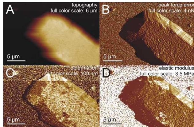
**FIGURE 3.** PF-QNM measurements on a lens nuclear cell. Topography (A), peak force error signal (B), deformation map (C), and elasticity map (D) measured concomitantly. Please note the fine surface structure visible in A and B.
