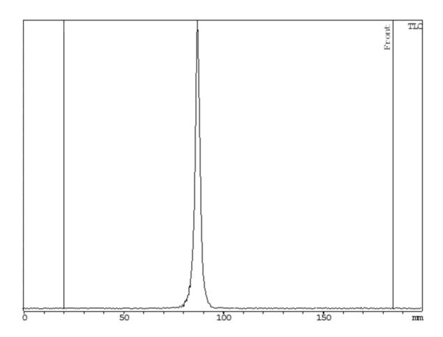
**2B:** Analysis of unlabelled AceDoPC by reverse phase high performance liquid chromatography (X Bridge  $C_{18}$  column) using a linear solvent gradient: solvent A and B were a mixture of methanol/water/acetonitrile (95/35/2.5 and 100/4/2.5, v/v, respectively) from 5 to 35 min (1ml/min). AceDoPC was detected at 205 nm after 27 min.
