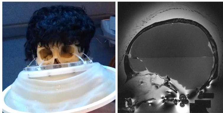
Figure 3 Skull with wig strapped to holder ( left ) and as seen on MR T2w sagittal image ( right ).
