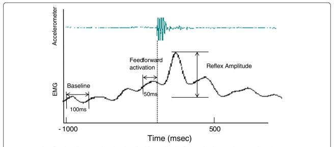
Figure 1 Sample reflex data illustrating how baseline, feed forward and reflex amplitude were determined. Baseline EMG activity was measured 1 second before perturbation during 100 ms. Feedforward activation was determined 50 ms before the perturbation. Reflex amplitude was quantified as the peak magnitude of normalized EMG.
