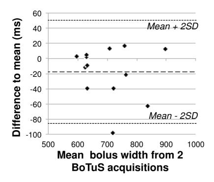
Figure 3: Repeatability of the BoTuS results shown in a Bland-Altmann graph representing the difference to the mean for two separate measurements as a function of their mean.
