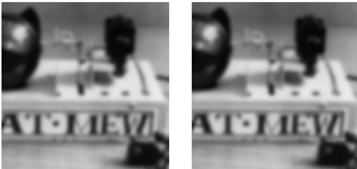
Figure 11 Smoothed image with [left] ITK's CPU Deriche recursive Gaussian smoothing filter (sigma=12) and [right] ITK's CPU discrete Gaussian smoothing filter (variance=144). (Single precision.)
