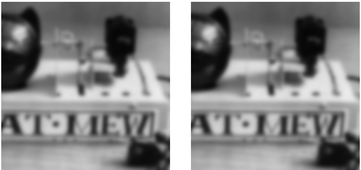
Figure 10 Smoothed image with [left] CPU and [right] GPU implementations, \sigma=12 . (Operations in single precision, float.)
