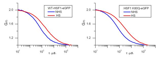
**Figure 6. FCS analysis of HSF1 -K80Q in immortalized MEFs form HSF1 null mice.** Dynamics of HSF1- K80Q-eGFP and WT HSF1-eGFP before (NHS, blue) and after 30 minutes heat shock (HS, red) in immortalized MEFs from HSF1 null mice. doi:10.1371/journal.pone.0067566.g006
