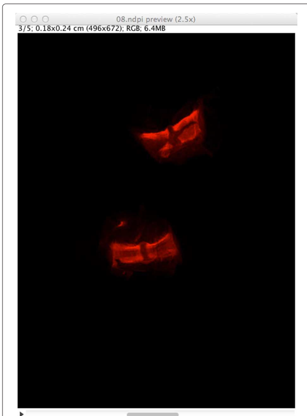
Figure 3 Preview image of a NDPI file with several focalization levels in ImageJ. The NDPI file 08.ndpi contains images at 5 different focalization levels. Therefore, its preview image is displayed as a stack of 5 images.
