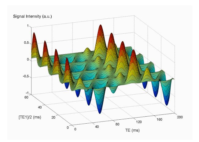
**Figure 2.** Simulated proton MR spectra of the citrate resonances at 11.7 T for the double spin echo sequence (PRESS sequence) and for the double spin echo sequence with the additional 180° pulse (gPRESS sequence). The sequence delays (total TE = 132 ms and TE<sub>1</sub> = 20 ms) are chosen to illustrate here the large effect of the 180° pulse on the spectral shape and signal intensity of the citrate resonances. The same vertical scale is used for both spectra.
