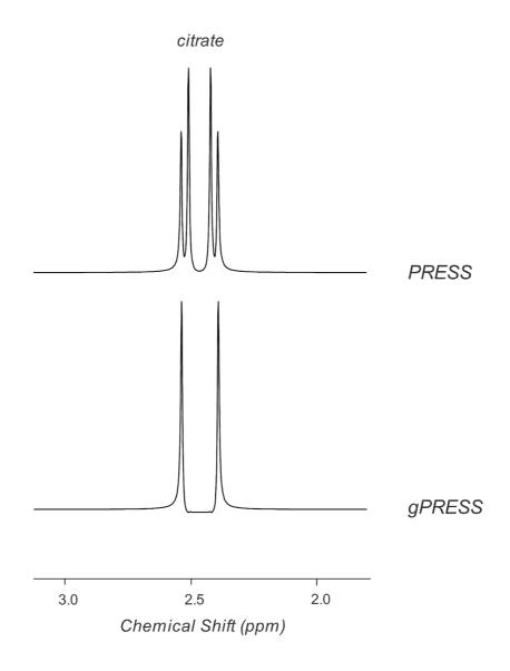
**Figure 3.** Spectra acquired at 11.7 T from a phantom containing citrate, lactate and glycine. The additional 180° pulse in the double spin echo sequence has a large effect on the citrate resonances, but no effect on the glycine (singlet) and lactate (weakly coupled) resonances. The sequence timings are TE = 132 ms and  $TE_1 = 20$  ms. The spectral shape of the citrate resonances agrees well with the simulated spectra shown in Figure 2.
