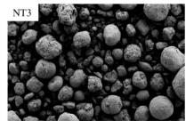
**Figure 1 SEM observations.** Representative scanning electron microscopy (SEM) image of uncoated multi-walled carbon nanotubes (NT1) and of the same nanotubes coated with carboxylic polyacid polymer (NT2) or polystyrene polybutadiene polymethacrylate polymer (NT3).
