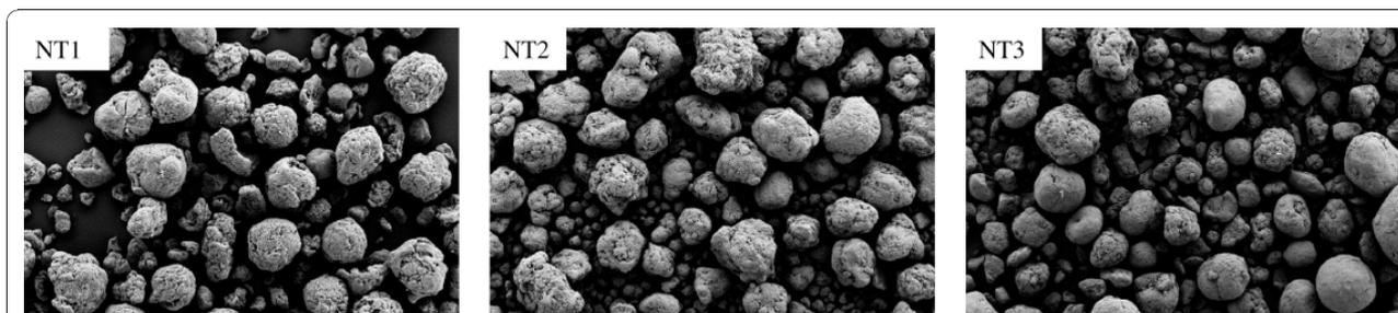
**Figure 1 SEM observations.** Representative scanning electron microscopy (SEM) image of uncoated multi-walled carbon nanotubes (NT1) and of the same nanotubes coated with carboxylic polyacid polymer (NT2) or polystyrene polybutadiene polymethacrylate polymer (NT3).
