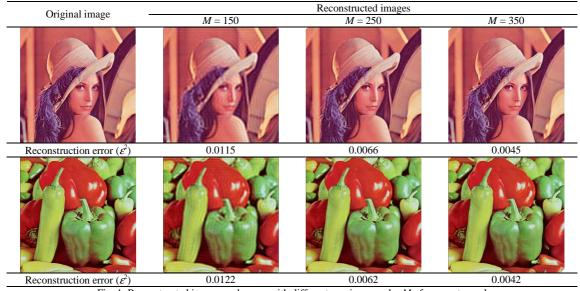
Fig. 1. Reconstructed images and errors with different maximum order M of moments used
