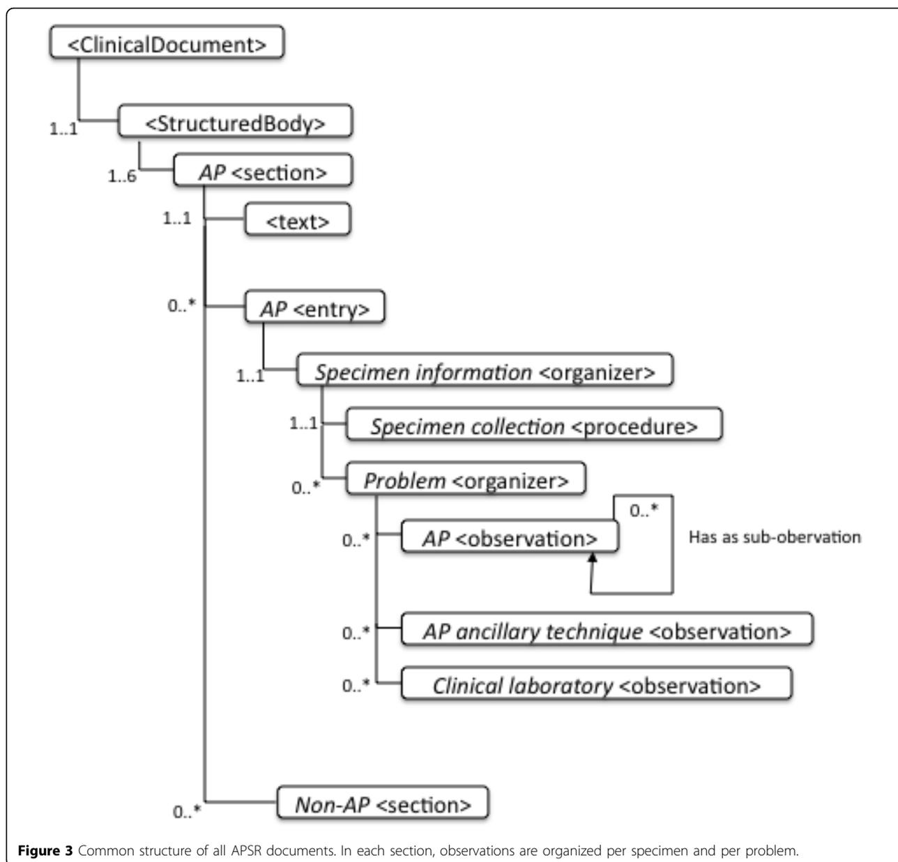
**Figure 3** Common structure of all APSR documents. In each section, observations are organized per specimen and per problem.
