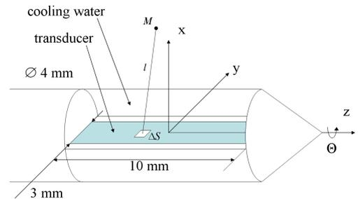
Fig. 1. Ultrasound device geometry and coordinates system.
