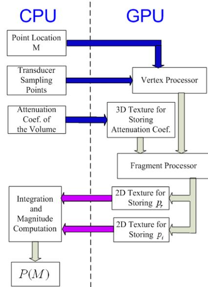
Fig. 2. Program flow chart of GPU-based Rayleigh integral.
