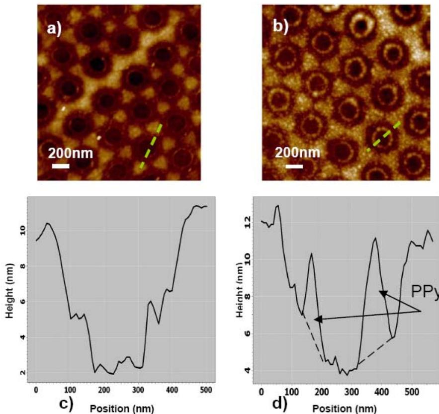
**Fig. (3).** AFM images and profiles comparing the SiO<sub>x</sub> nanotemplate nanoarrays before (a-c) and after (b-d) the PPy growth. a-c) topographic images, b-d) height profiles along the dot lines. (c)-(d) vertical scale 0-20 nm.
