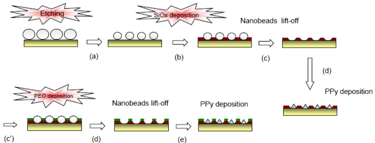
**Fig. (1).** Scheme of the production of the gold/SiO<sub>x</sub> nanotemplate (a) Plasma etching of the PS beads (b) PE-CVD deposition of SiO<sub>x</sub> layer, (c') PE-CVD deposition of PEO layer, (c) and (d) lift-off of the beads, (d') and (e) polypyrrole deposition by electro-co-polymerisation.
