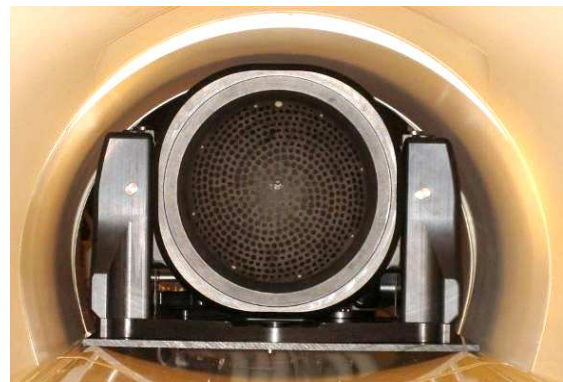
Figure 4. HiFU device for brain tumor therapy compatible with MRI. General view (left), device (right). Courtesy Mickael Tanter, Mathias Fink (Tanter, Thomas et al. 1998; Aubry, Tanter et al. 2003; Tanter, Pernot et al. 2007).
