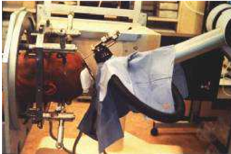
Figure 8. The pioneering robot, IGOR, designed by S Lavallée and P Cinquin, TIMC, in 1989, for brain biopsy (stereotactic frame on the left, robot arm on the right, with X-ray guidance of the needle, middle)
