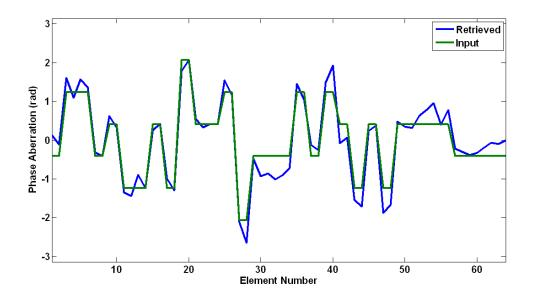
Figure 9. Numerical phase aberrations along the 64 elements linear array: programmable phase aberrations (green curve) and recovered values for the MR guided experiment with MSG frequency at 600Hz (blue curve).
