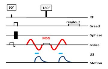
Figure 3. Proposed MR sequence for radiation force imaging at 7T. Two 600Hz sinusoidal gradients are added on the slice selection axis of a standard spin echo sequence. Two 400µs US pulses are triggered to the second lobe of each of the MSG.
