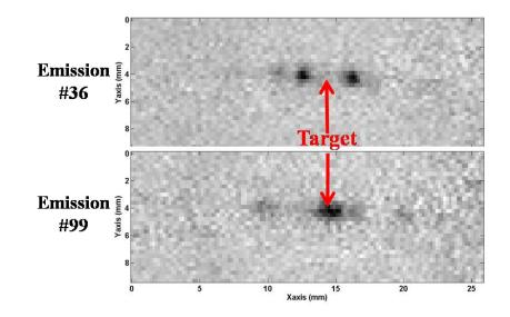
Figure 8. Example MR phase images for two Hadamard coded emissions (#36 and #99) in the presence of a programmed aberration in front of the ultrasonic array.
