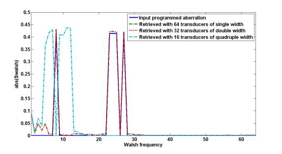
Figure 16. Walsh spectrum of the programmed aberrator together with the spectra of the aberrators retrieved from the simulated experiments with 64 0.3mm width elements, 32 0.6mm width elements and 16 1.2mm width elements.
