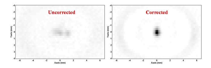
Figure 14. Measured MR phase maps in the focal plane (XY) prior any correction (left) and after the adaptive focusing procedure (right).
