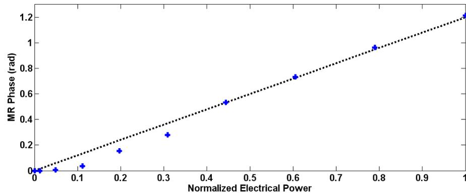
Figure 4. Calibration curve obtained with a PDMS physical aberrator in front of the linear array. The MR phase is plotted as a function of the normalized electrical power together with the best linear fit. All subsequent acquisitions were performed at maximum power.
