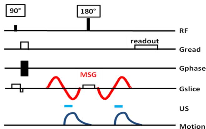
Figure 3. Proposed MR sequence for radiation force imaging at 7T. Two 600Hz sinusoidal gradients are added on the slice selection axis of a standard spin echo sequence. Two 400 $\mu$ s US pulses are triggered to the second lobe of each of the MSG.
