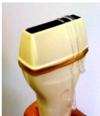
Figure 11. Picture of the ultrasonic linear array with two PolyDiMethylSiloxane stripes positioned in front of it to generate strong aberrations.
