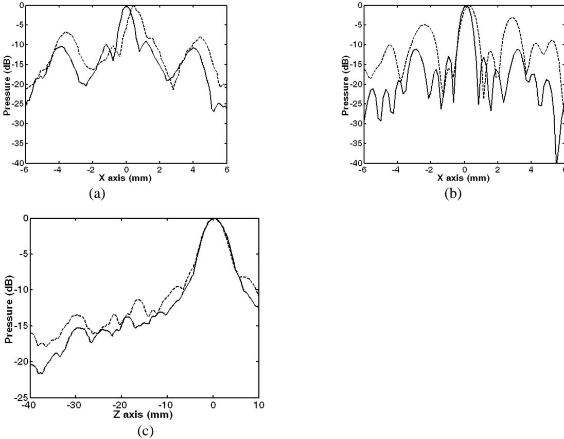
**Figure 7:** Pressure distribution (dB scale) obtained with time reversal (gray line) and with no correction (dotted line) in the focal plane (a: experiment and b: simulation) and along the beam axis (c: experiment).
