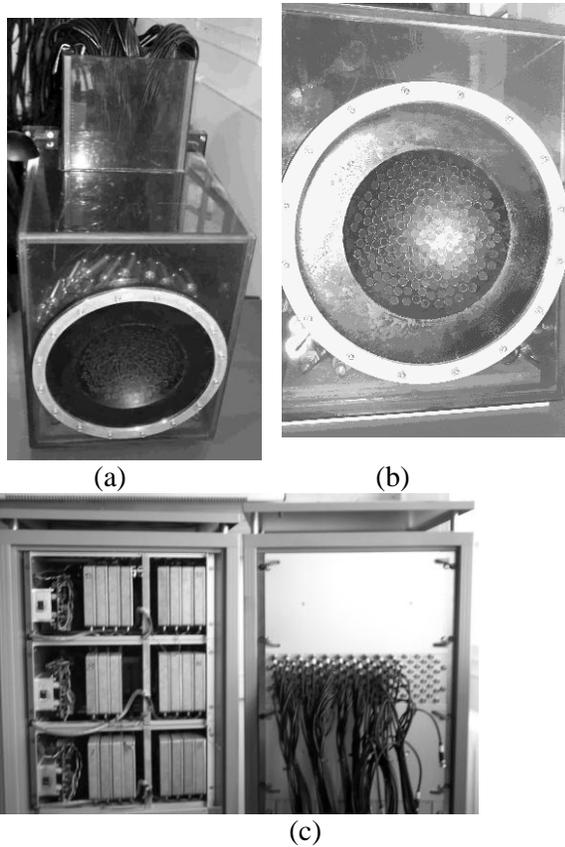
**Figure 1:** 200 elements sparse array prototype and the electronic system. (a) The waterproof plastic box contains the 200 electrical matching boxes. (b) Front view of the array: the transducers are mounted on a spherical surface. (c) High Power electronics (individual channels)
