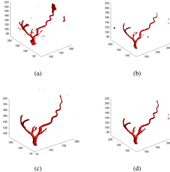
Fig. 4. Influence of the relaxation value in the quality of the reconstruction: (a) $\sigma=0.5$  (MSE:16.27%), (b) $\sigma=0.6$  (MSE :8.93%), (c) $\sigma=0.7$  (MSE: 2.55%) (d) $\sigma=0.8$  (MSE :4.35%)
