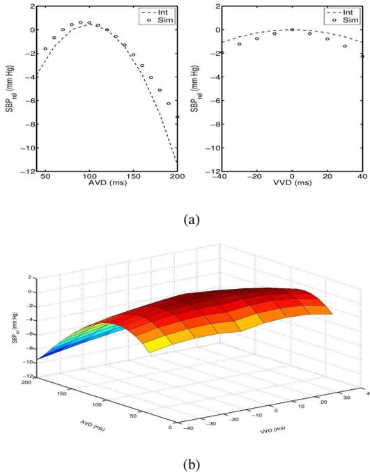
Figure 6. (a) Comparison between interpolated clinical data (dash) and simulation results (circles) for  $SBP_{rel}(AVD)$  at  $VVD = 0$  ms (left) and  $SBP_{rel}(VVD)$  at  $AVD = 120$  ms (right) for an optimal configuration of  $AVD = 100$  ms and  $VVD = 0$  ms and (b)  $AVD/VVD$  scanning results of the simulations.
