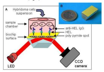
Figure 1. (A) Scheme of the SPR imaging setup.(B) Photograph of a gold-coated chip.
