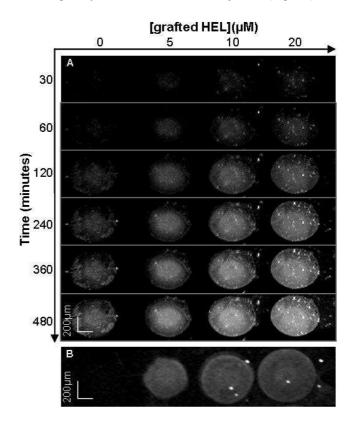
Figure 2. (A) SPR image of a biochip containing HEL spots (5, 10 or  $20\mu M$ ) or cytochromeC control spot (HEL  $0\mu M$ ) after different times of exposure to secreting cells. (B) Image of the same spots observed at the end point of the experiment by fluorescence microscopy after staining with antimouse IgG (Fc specific).
