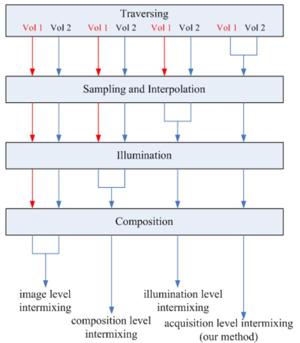
Figure 1: Rendering pipeline for different intermixing levels
