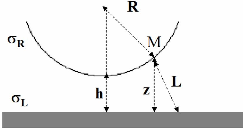
**Figure 5 : Counting the number of ligand-receptor couples interacting in the flow chamber.** Defining as  $L$  the range of the interaction, a point  $M$  of the microsphere surface can interact with ligand molecules located on a disk of area  $\pi(L^2 - z^2)$  on the chamber floor.
