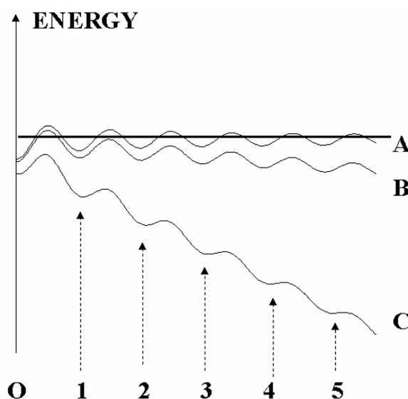
**Figure 6 : Difficulty of defining binding states.** A unidimensional energy landscape is shown, revealing a series of binding states of decreasing depth (numbered 0, 1 ...5), as illustrated by curve A. The "overall" bound state must be defined somewhat arbitrarily. Applying a growing disruptive forces (curves B and C) will flatten the energy barriers, and the weakest complexes will disappear (see e.g. 5 on C).
