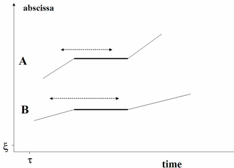
**Figure 4 : Calculated arrest duration is dependent on arrest definition.** The thick lines represent binding events of equal length separating two periods of more rapid (A) or slower (B) displacement. The broken lines show the periods of time where particles are defined as arrested, using threshold parameters  $\xi$  and  $\tau$  as defined. Clearly, a correction is required to obtain "true" arrest duration.
