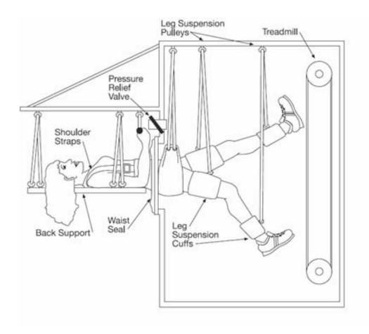
**Figure 1**. Exercise on a treadmill within lower body negative pressure (LBNP) exposure. Footward force is produced by the pressure gradient generated by LBNP. The subject is suspended at the ankles and thighs by a pulley system, and the hands are holding the suspension cables at waist level.
